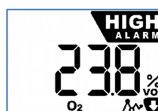
Alarm Value Occurred Display
