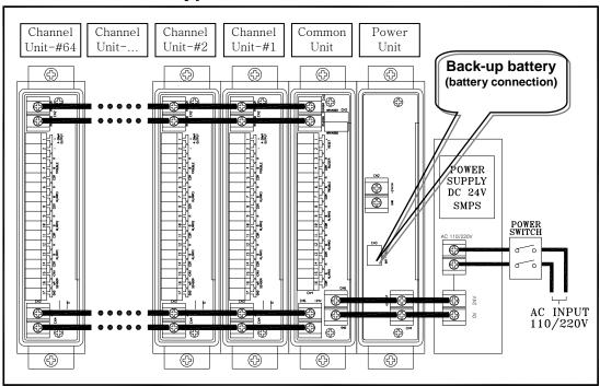
\*. Power Unit is supplied only when using Battery. In case of no Power Unit, DC power (24V) is directly connected from Power Supply to connector (CN6) of common unit. (Power Unit is an option item.)
