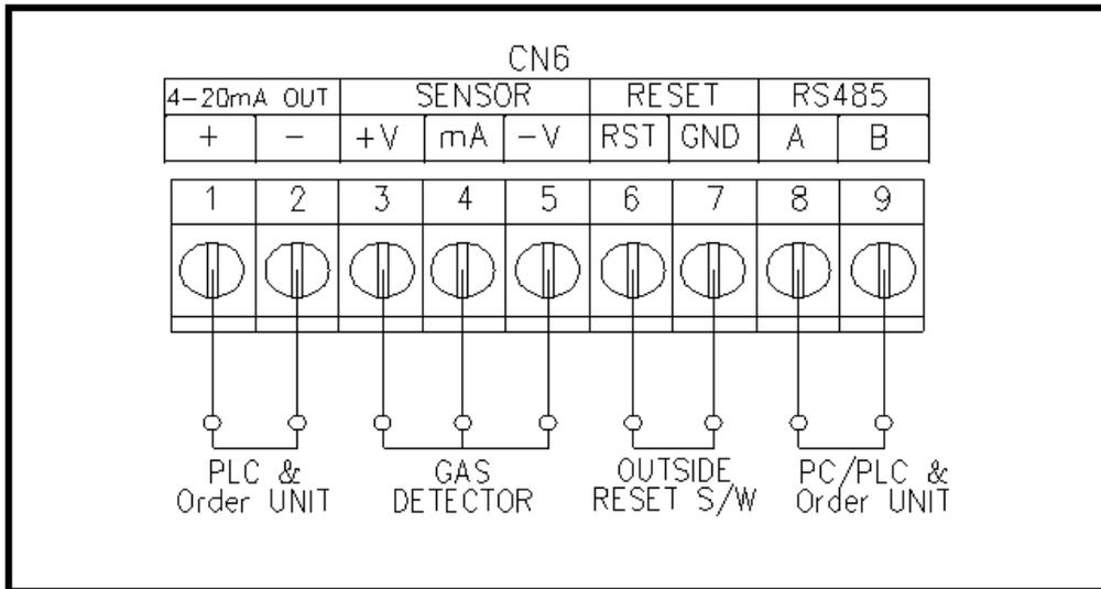
*Caution) RS-485 Cable should be used dedicated RS-485 cable and for the connection cable to connect with 4~20mA output and detector, the shield cable of CVVS or CVVSB higher than 0.75sq should be used!*
