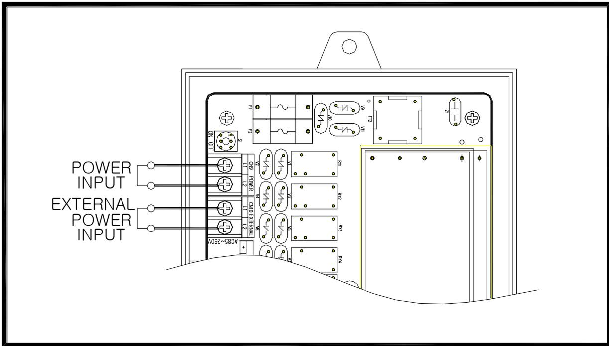
Connect the AC power (85~260V 50/60Hz) to CN7 as shown in figure.
