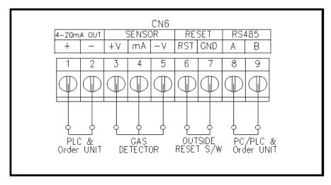
Caution) RS-485 Cable should be used dedicated RS-485 cable and for the connection cable to connect with 4~20mA output and detector, the shield cable of CVVS or CVVSB higher than 0.75sq should be used!
