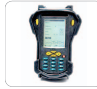
HAND-HELD DIAGNOSTIC KIT Certified I.S. (EExia) for use in the hazardous area and connects to I.S. port on 900.
